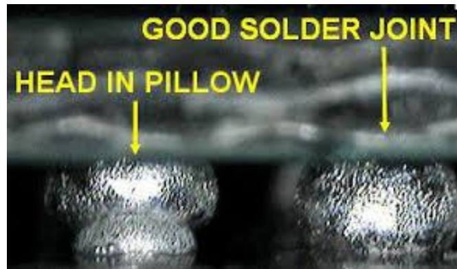
Figure 7. Head-in-Pillow Defect Compared with a Good Solder Joint
